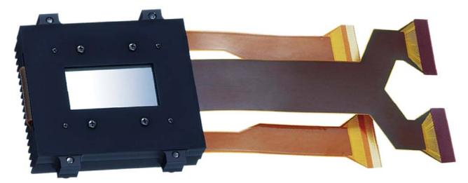
More than 8 megapixels on an inch and a half of silicon, this is Sony's 4K SXRD panel. The four input ribbons correspond to the projector's four input slots and the four 2K quadrants of the panel.
